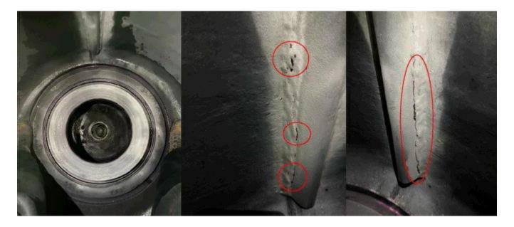
Main steam stop valve seat. Weld cracking identified with red circles.
